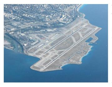
There are one set of close parallel runways; one is the runway (04L/22R) 2,570m and the other is the runway (04R/22L) 2,960m. There are two terminal buildings; Terminal 1 (52,000 m<sup>2</sup>) has 25 gates with a capacity of 4.5 million passengers, Terminal 2 (57,800 m<sup>2</sup>) has 29 gates with a capacity of 8.5 million passengers.
